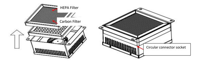
3.After changed filters, Located the air purifier, and tighten the 4pcs screws, Special notes: the Aviation sockets of air purifier must be toward the back of oven!
